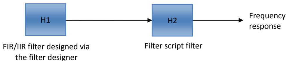
As seen, the main FIR/IIR filter designed via the filter designer GUI is assigned to the *primary filter*, H1. All poles and zeros defined via the filter script are added to a *secondary filter block*, H2. The H2 filter block implements the filter as a single section (i.e. no biquads) IIR, which eases the implementation, but also the advantage of assigning poles to an FIR primary filter. In the case of no poles, the H2 filter becomes an FIR filter.
