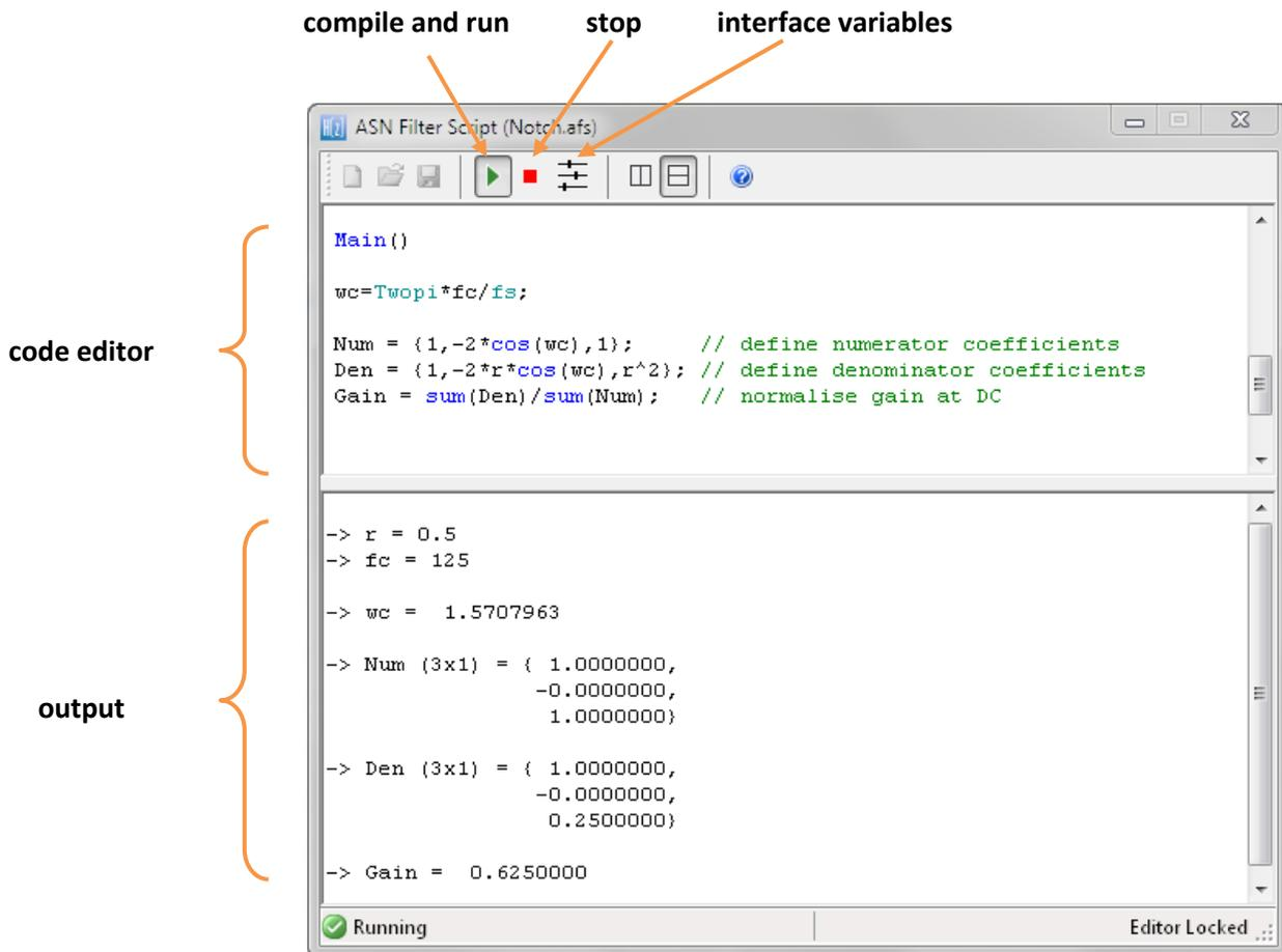
As seen, the IDE is split up into a code editor and an output window. The IDE differs from other scripting IDEs in that all executed code appears in the output window, and there is no provision for entering and evaluating expressions in the output window directly.
