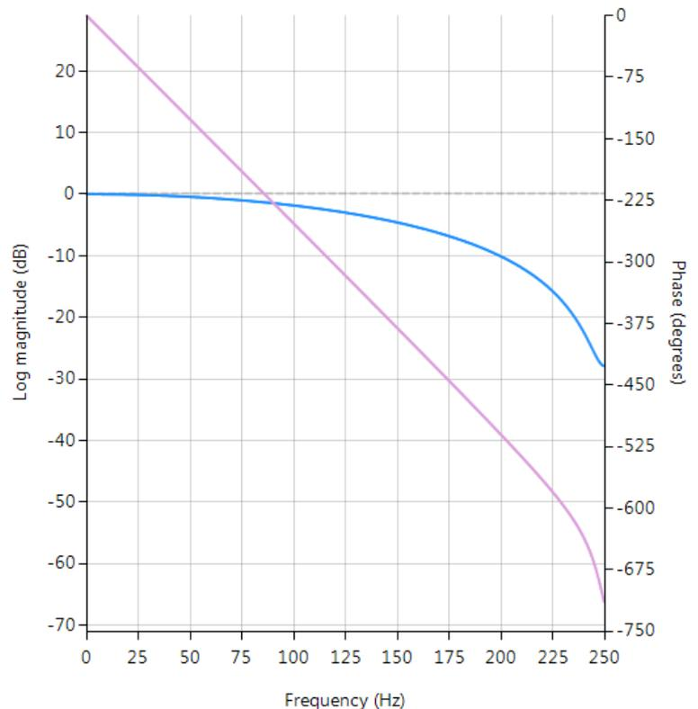
The plot shown on the right shows the magnitude (blue) and phase (purple) spectra for  $\Delta = 9, \alpha = 0.52$ . As seen, the fractional delay element results in a non-flat magnitude spectrum at higher frequencies.
